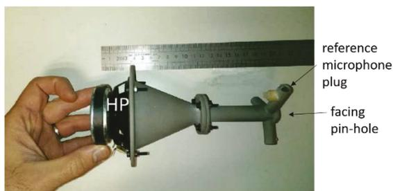
Figure 3-7 - Typical device for the calibration of RMPs or similar pin-hole wall-pressure sensors. The tripod end ensures right surface positioning.
